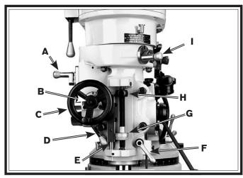
Figure 39. Fine downfeed controls.
